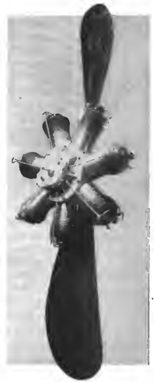
Gnome 7-Cylinder Motor, Used by Farman.
